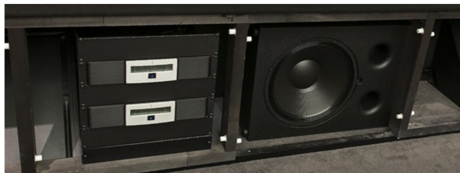
While the main equipment rack is outside the cinema room to minimise noise, light and heat, the Pro Audio Technology amplifiers for the front speakers and subs are at the front of the room, in the small rack shown above. “The reason is that we use balanced XLR cables to allow the signal to travel long distances with no loss,” says David Moseley. “But speaker cable works best when the cables are as short as possible. The surround channels are just as close to the rear rack, so we put the amps there for those speakers.”
